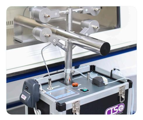
Designed to meet the test specification in BS.EN12469:2000 as a method for measuring operator and aperture protection factors in Class I and Class II microbiological safety cabinets.
