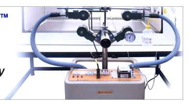
**KI-DISCUS MK2** - Designed to meet the test specification in BS.EN12469:2000 as a method for measuring operator and aperture protection factors in Class I and Class II microbiological safety cabinets.
